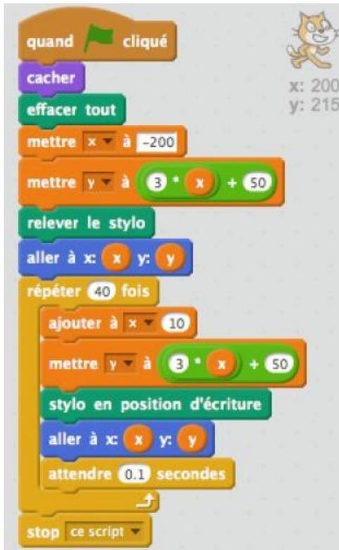
Scratch script for Exercise 3. The script starts with a 'when clicked' event, followed by 'hide', 'clear all', and 'set x to -200'. Then, 'set y to 3 \* x + 50' is used. The pen is lifted, and the cursor moves to (x, y). A loop repeats 40 times, adding 10 to x, recalculating y as 3 \* x + 50, setting the pen to drawing position, moving to the new (x, y), and waiting 0.1 seconds. The script ends with 'stop this script'.
